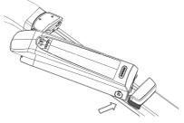
3. Push the battery into the battery holder, when hears a 'click' sound, that means battery is locked.
